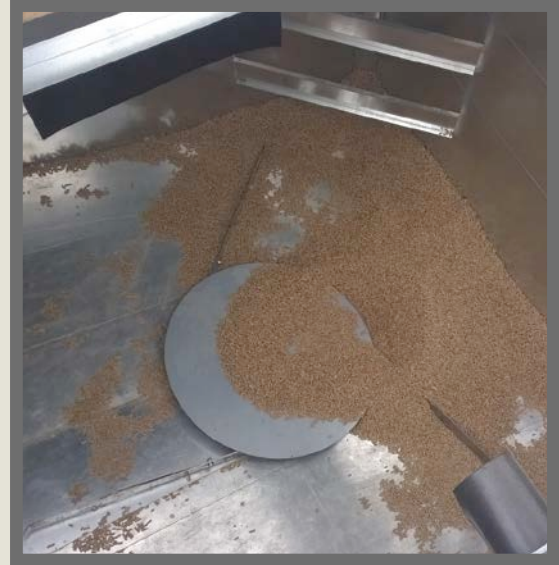
Steel Silo Base – Manufactured to suit extraction system.
